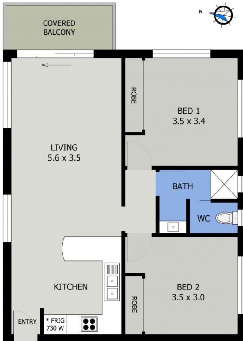
FLOOR PLAN ( 67 sq m Approx ) ( Scale: 1:55 )
