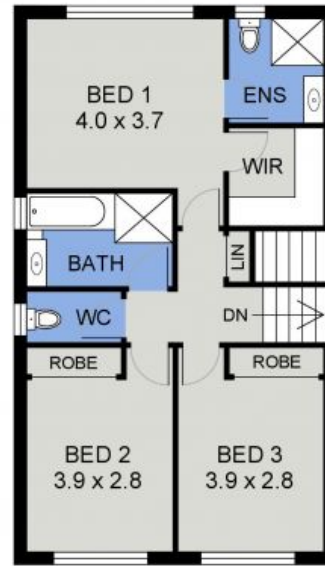
UPPER FLOOR PLAN (65 sq m Approx)
