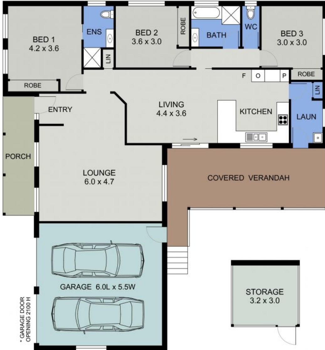
FLOOR PLAN (175 sq m Approx) Scale - 1:90
