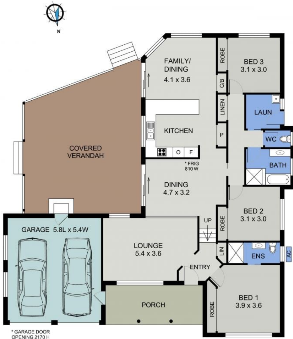
FLOOR PLAN (180 sq m Approx) Scale - 1:90
