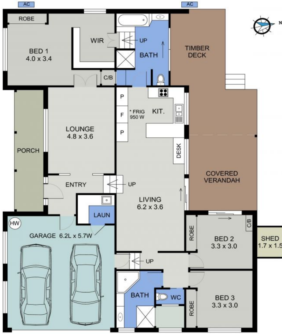
FLOOR PLAN (185 sq m Approx) Scale - 1:90
