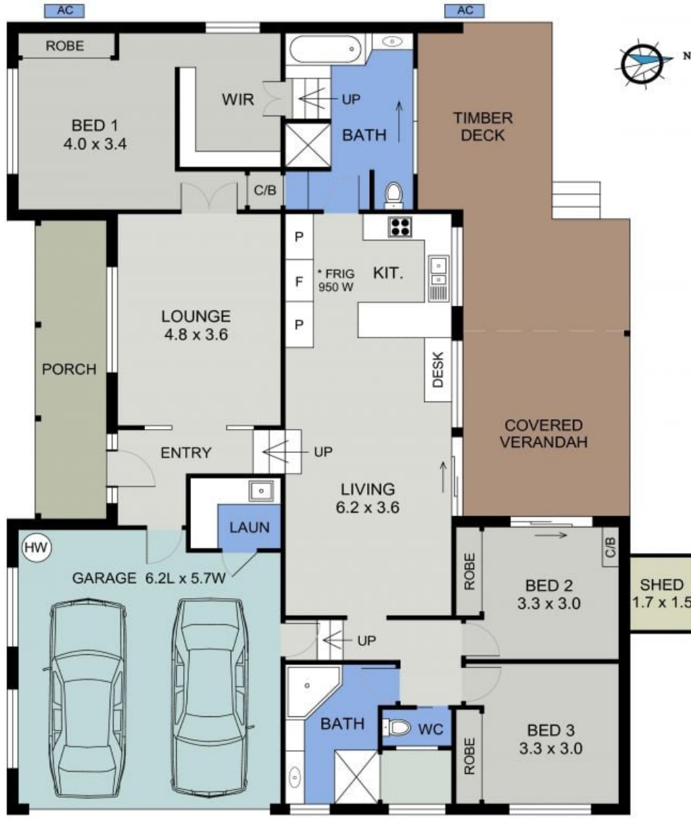
FLOOR PLAN (185 sq m Approx) Scale - 1:90
